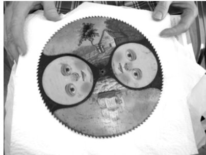
Iain MacDonald showed the group the dial he repaired (the dial belongs to John Ruhland). The brass of the dial was corroding underneath the paint. Iain 'filled in the gaps', making a beautifully restored dial. Iain has offered this service to others, for a fee.
