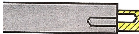
Figure 2, above, shows the inserted plug with the material needing removal shown in yellow
